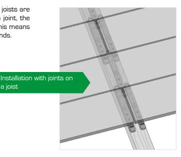
Ensure that the boards are positioned correctly. Ensure that the fasteners are positioned correctly under boards without joints so as not adversely affect the positioning of the fasteners on adjoining boards.
