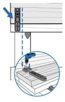
Position the cleats at the edge of the new board according to the diagram. Fix with screws.
