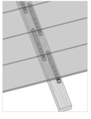
Sketch of fasteners under boards for an installation without adjoining boards.
