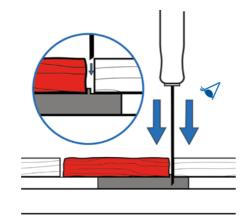
Locate the fasteners with stop tabs on the underside of the damaged board.
